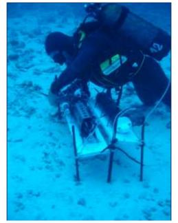
**Figure 3.** View of the data logger as set out on the reef to collect environmental parameters.
